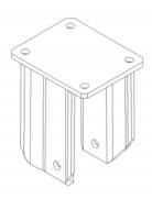
Medium-heavy duty bracket type EP (max. carrying capacity 1600 daN)
