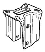
The bracket is made by a galvanised steel fork.
