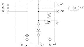
The pressure for unclamping must be at least 20% of the clamping pressure.
