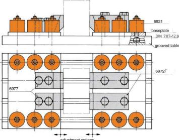
The shown hydraulic clamping device shows casts of several sizes that are clamped by hydraulic pull-down clamp no. 6972F and pull-down counterpart no. 6977. To obtain an efficient means of adjustment, 2 base plates are each equipped with 6 hydraulic nuts no. 6921 which are connected to the grooved table via bolts for T-nut according to DIN 787. The adjustment of the base plate and the clamping of the workpiece can be performed independently by a pump unit with 2 clamping circuits.
