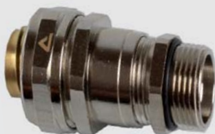
ISO cable-hose fitting, compact, male, double seal acc. EN 45545-2, HL1 / HL2 / HL 3, table R22 and R23 (incl. brass connection set)
