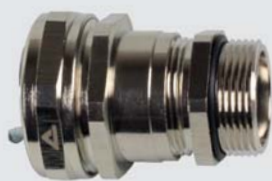
ISO cable-hose fitting, compact, male, double seal acc. EN 45545-2, HL1 / HL2 / HL 3, table R22 and R23 (incl. metal clamping ring)
