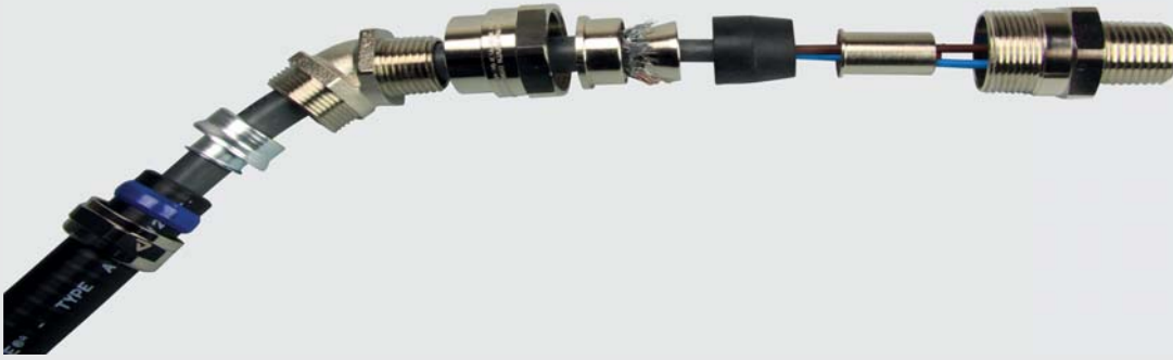
BAC, ISO, IECEx-ATEX EMC cable-adapter, nickel plated brass, EPDM and epoxy seal (-40 °C till +100°C)
