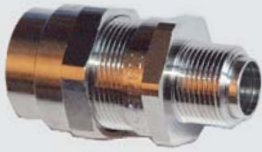
BAC, ISO, IECEx-ATEX EMC cable-adapter, nickel plated brass, EPDM and epoxy seal (-40 °C till +100°C)
