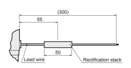
The alternating current (AC) type has a rectification stack assembled into the lead wire.
