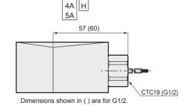
Stainless steel body + grommet lead wire type AG44-02/03-1 to 4-D/E/L/M/R
