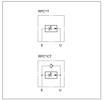
**RPC\*** PRESSURE AND TEMPERATURE COMPENSATED FLOW CONTROL VALVES
