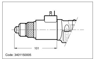
12.3 - CPK Push manual override with mechanical retention
