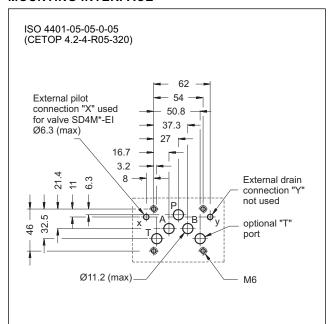
The internal pilot version of the valve can be installed either on the ISO 4401-05 (CETOP 05) type or ISO 4401-05-05-0-94 (R05) type of mounting interface (ports X and Y of the latter version are not to be used).
