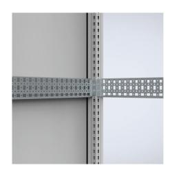
**Description:** Universal profile for both depth and width fitting on the 25 mm DIN hole pattern on the enclosure frame. The 75 mm wide profile is equipped with three rows of holes of which one is turned  $90^{\circ}$ . This makes it possible to mount the CLPO profiles in both directions. The CLPO increases the useful space by 25 mm.
