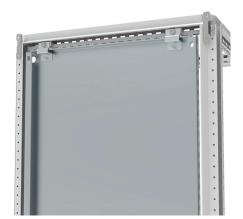
**Description:** To fix mounting plates to the enclosure from rear. The kit includes brackets for fixing the mounting plate flush with the enclosure frame or set back behind the enclosure frame, adding +20mm of useful depth for mounting components. These brackets are needed when rear fixation is required or when the enclosure is ordered without the mounting plate (PE) as an alternative to MPA06/MPA04. Unmounting from both the front and rear is possible.
