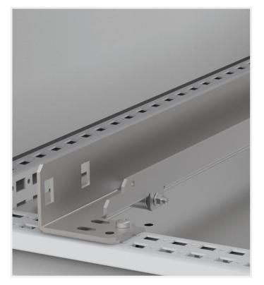
The roller reduces the friction between sliding profile, MTS and mounting plates, MPW/MP, reducing the force to be applied during the side-mounting, specially for heavy loaded configurations. Item no. MTS01W
