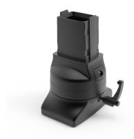
**Additional information:** The flange coupling attaches a tube to the enclosure, enabling 300-degree enclosure rotation and can be locked into a given position. The flange coupling has a safety stop and maintenance-free bearings. Die-cast aluminum construction. Includes installation instructions, gaskets, tube setscrews and enclosure mounting hardware.
