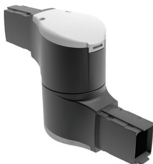
**Additional information:** Use an intermediate joint to join two horizontal tubes together for a longer length. The arm can be rotated 300 degrees. Includes safety stop and maintenance-free bearings. Die-cast aluminum construction. Includes installation instructions, gaskets, and tube setscrews. Use of the intermediate joint reduces the system load rating capacity to 146 lb. (66 kg) at 3.3 ft. (1 m).
