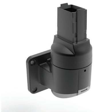
**Additional information:** The vertical wall joint mounts the suspension system to a vertical surface, allowing the tube to extend vertically. The arm can be rotated 300 degrees. Includes a safety stop and maintenance-free bearings. Die-cast aluminum construction. Includes installation instructions, gaskets, and tube setscrews. Surface mounting hardware is not provided.
