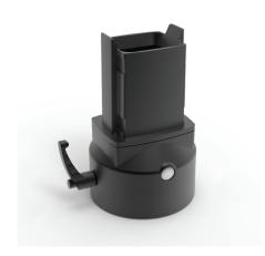
**Additional information:** Flange Coupling attaches a tube to the enclosure, enabling 300-degree enclosure rotation. The enclosure can be locked in position. Flange Coupling has safety stop and maintenance-free bearing. RAL 9005 black finish. Die-cast aluminum construction. Includes installation instructions, gaskets, tube setscrews and enclosure mounting hardware.
