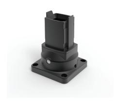
**Additional information:** Rotary Base allows the entire suspension system to rotate at the point of attachment on a horizontal surface. The arm can be rotated or turned 300 degrees. Includes safety stop and maintenance-free bearing. RAL 9005 black finish. Die-cast aluminum construction. Includes installation instructions, gaskets and tube setscrews. Surface mounting hardware is not provided.
