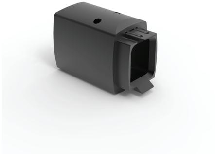
**Additional information:** Use a Tube Adapter when the tube is cut to length and it is not desirable to drill and tap new holes in the tube. The adapter attaches to the tube with internal setscrews and provides mounting holes at the end where the tube was cut. RAL 9005 black finish. Die-cast aluminum construction. Includes installation instructions, gasket and hardware for attaching to the tube.
