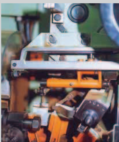
Picture 5.1: By converting to iglidur® W300 the life of the bearing on this tea bag packaging machine was increased by five times
