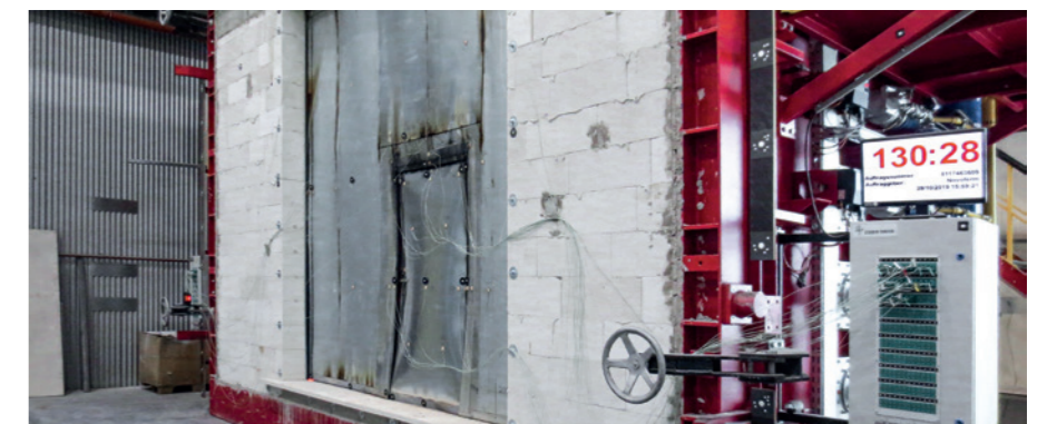
Fire test, view after 130 minutes
