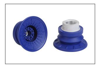
Size: 50 Suction cup material: Nitrile rubber NBR Material hardness: 60 °Sh Vacuum connection: G3/8"-F Nipple material: Aluminium Number of folds: 1.5
