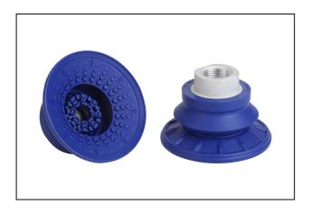
Size: 60 Suction cup material: Nitrile rubber NBR Material hardness: 60 °Sh Vacuum connection: G3/8"-F Nipple material: Aluminium Number of folds: 1.5
