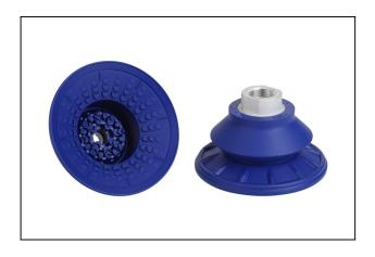
Size: 80 Suction cup material: Nitrile rubber NBR Material hardness: 60 °Sh Vacuum connection: G3/8"-F Nipple material: Aluminium Number of folds: 1.5
