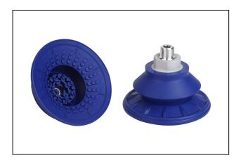
Size: 80 Suction cup material: Nitrile rubber NBR Material hardness: 60 °Sh Vacuum connection: G1/4"-M Nipple material: Aluminium Number of folds: 1.5
