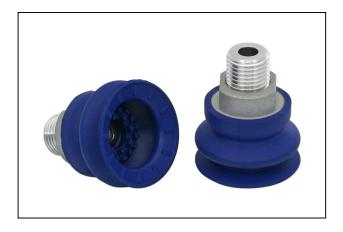
Size: 30 Suction cup material: Nitrile rubber NBR Material hardness: 60 °Sh Vacuum connection: G1/4"-M Nipple material: Aluminium Number of folds: 1.5
