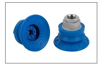
Size: 50 Suction cup material: High temp material HT1 Material hardness: 60 °Sh Vacuum connection: G1/4"-F Number of folds: 1.5 Nipple material: Brass, nickel-plated
