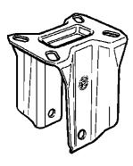
The bracket is made by an electrolytically galvanised steel fork.
