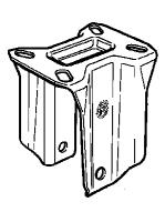
The bracket is made by a yellow galvanised steel fork.
