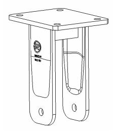
The bracket is made by a steel forged fixing plate with 4 holes, by two steel drawn sides and by a steel central stiffening. These elements are bounded by welding and properly protected against oxydation.
