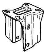
The bracket is made by an electrolytically galvanised steel fork.
