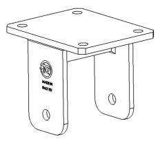
The bracket is made by a steel forged fixing plate with 4 holes, by two steel drawn sides and by a steel central stiffening. These elements are bounded by welding and properly protected against oxydation by electrolitycally galvanisation.
