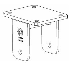
The bracket is made by a steel forged fixing plate with 4 holes, by two steel drawn sides and by a steel central stiffening. These elements are bounded by welding and properly protected against oxydation by electrolitycally galvanisation.
