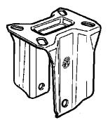
The bracket is made by a yellow galvanised steel fork.
