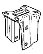
The bracket is made by AISI 304 stainless steel fork.
