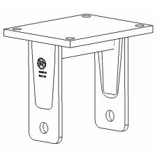
The bracket is made of a steel forged fixing top plate with 4 holes, of two steel drawn sides and of a central steel stiffener. These elements are secured by welding and properly protected against oxydation.
