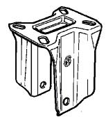
The bracket is made of AISI 304 stainless steel fork.
