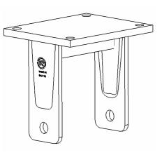
The bracket is made by a steel forged fixing plate with 4 holes, by two steel drawn sides and by a steel central stiffening. These elements are bounded by welding and properly protected against oxydation.
