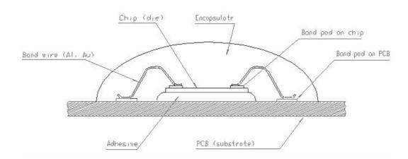
Above;the silicon chip is glued directly to the substrate and then connected by bonding with an aluminum wire or a gold wire with a diameter from 17.5 to 50 µm (no exhaustive list). An encapsulation resin (Glop top) can be dispensed on the unit or locally to guarantee stability against thermal and mechanical efforts, and to protect the assembly.
