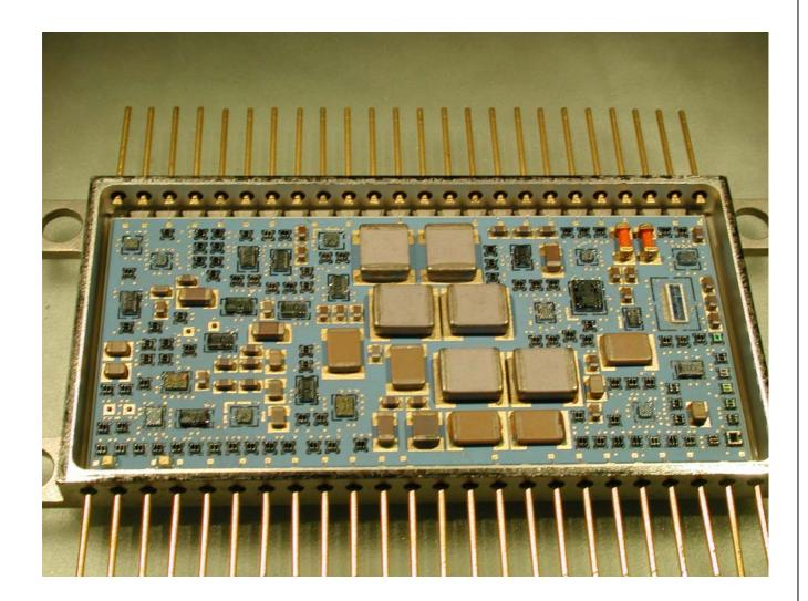
The manufacturing stages interconnects some passive components such as resistors printed on a ceramic substrate. With Hybrid technology several importants aspects may be taken to satisfy the requirements such as track width, proximity of tracks to bonding pads, bondability, loop heights, heat dissipation and so on must be con-sidered.
