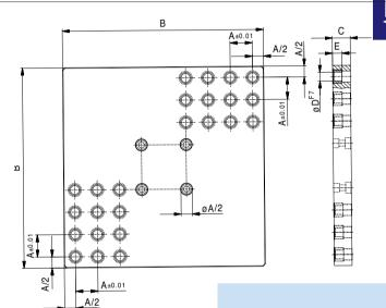
Unmachined base plates for jacks
