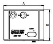
Operation via 220V power pack, integrated on/off switch with light display, vacuum switch and manometer.
